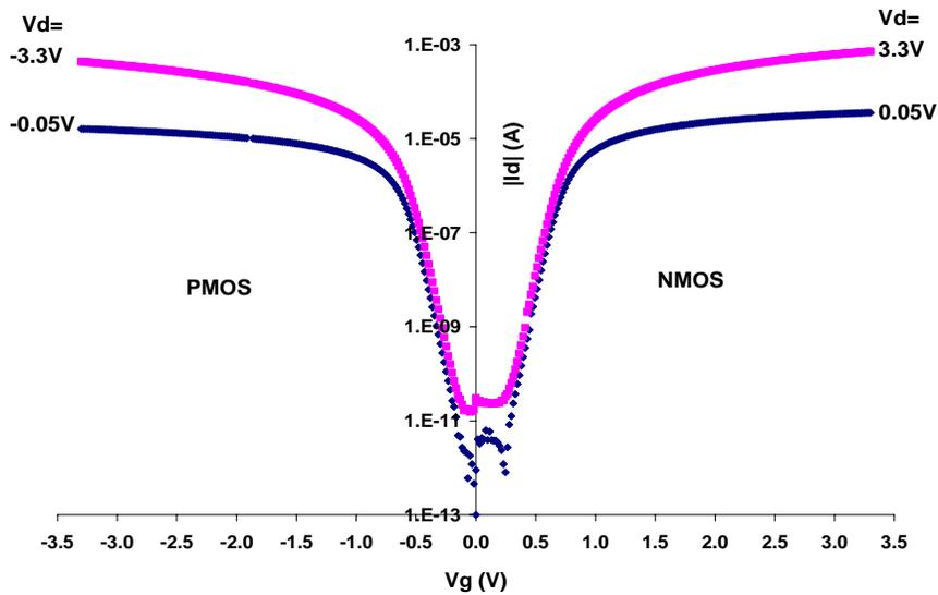
Fig. 16 - PMOS and NMOS sub-threshold characteristics
