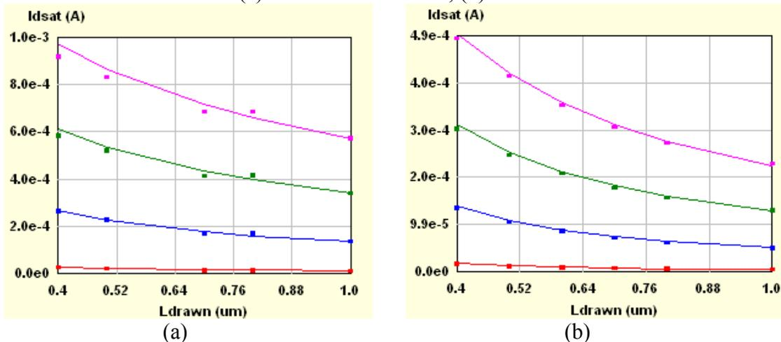
Fig. 24 - Saturation current vs. channel length at  $V_{bs}=0\text{V}$  with gate bias
