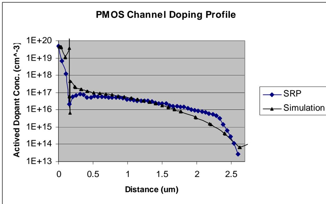
Fig. 8 - Simulated PMOS channel doping profile vs. SRP result
