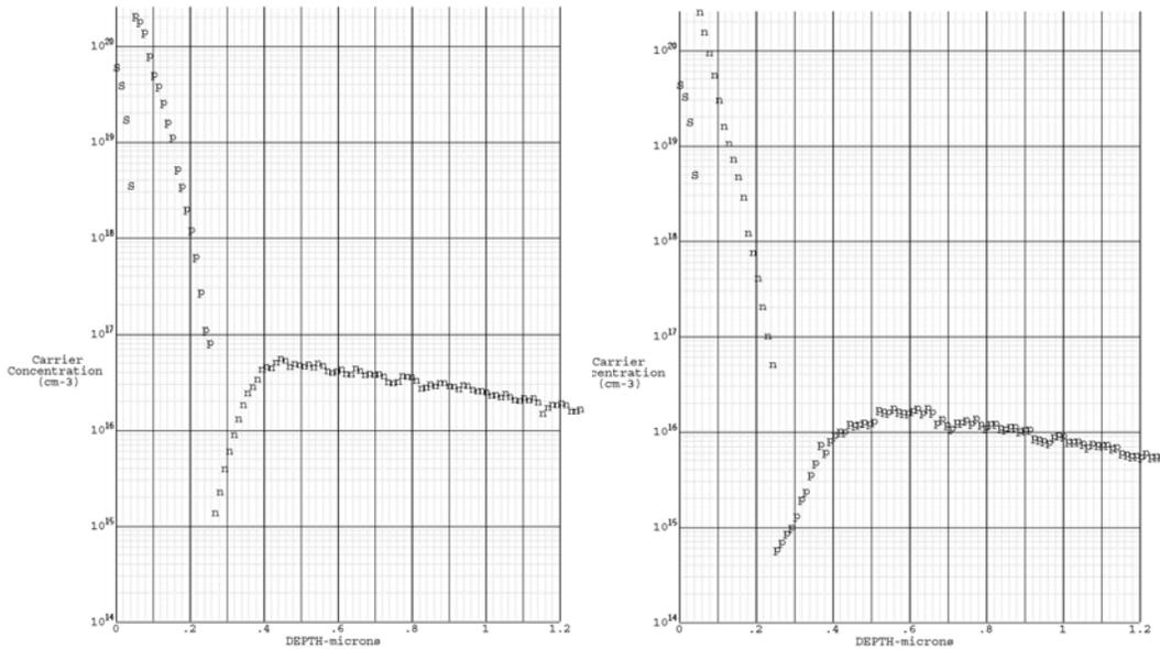
Fig.14 - P+ source-drain (left) and N+ source-drain doping profile
