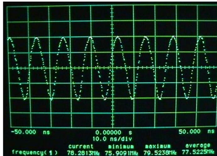
Fig. 21 – Snapshot of the oscilloscope screen showing 1 $\mu$ m gate ring oscillator frequency
