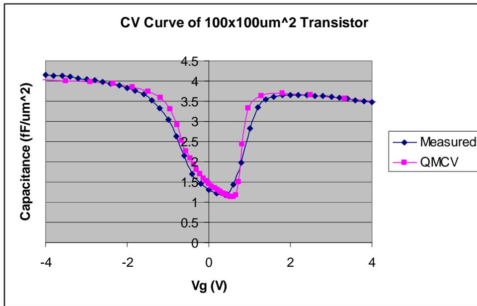
Fig. 10 - Measured and simulated CV curves of NMOS transistor (W/L=100/100) (Fitting parameters:  $t_{ox} = 8\text{nm}$ ,  $N_{poly} = 2E19$ ,  $N_{sub} = 2.1E17$ ,  $V_{fb} = -0.75$ )
