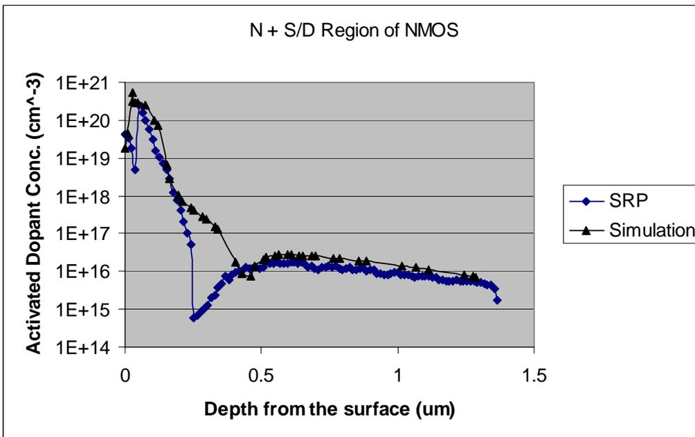
Fig. 7 - Simulated S/D junction profile of NMOS vs. SRP result
