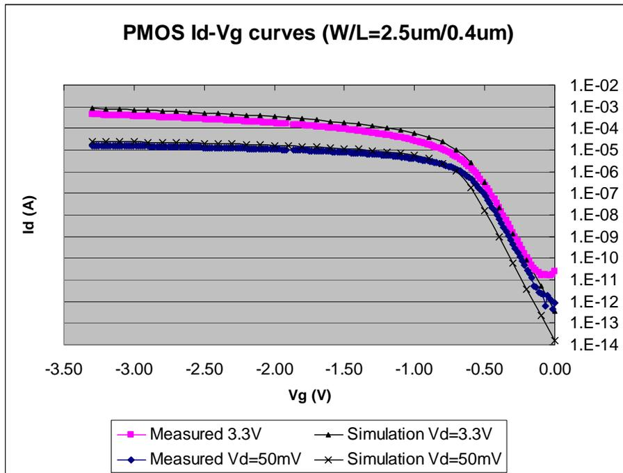
Fig. 11 - Measured and simulated Id-Vg curves of PMOS transistor (W/L=2.5/0.4)
