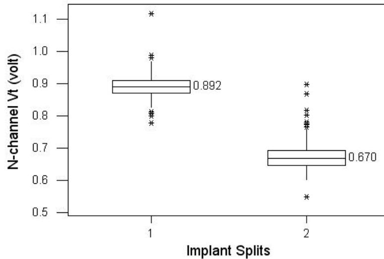
Fig. 19 - Threshold voltages in NMOS split groups:
