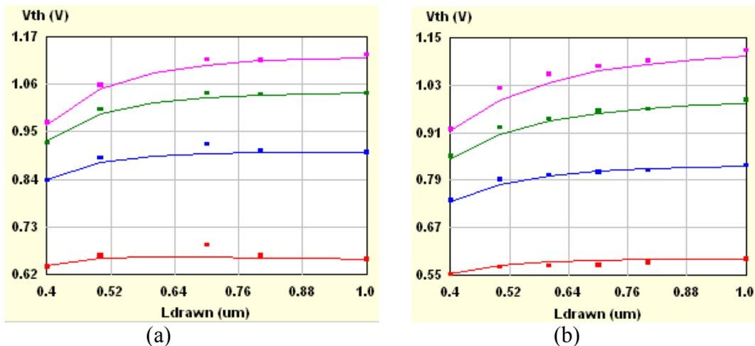
Fig. 23 - Threshold voltage vs. drawn channel length at  $W=2.5\mu\text{m}$  with substrate bias
