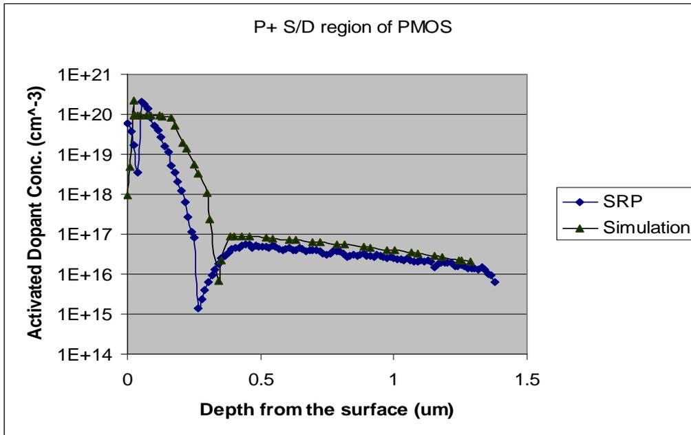
Fig. 6 - Simulated S/D junction profile of PMOS vs. SRP result
