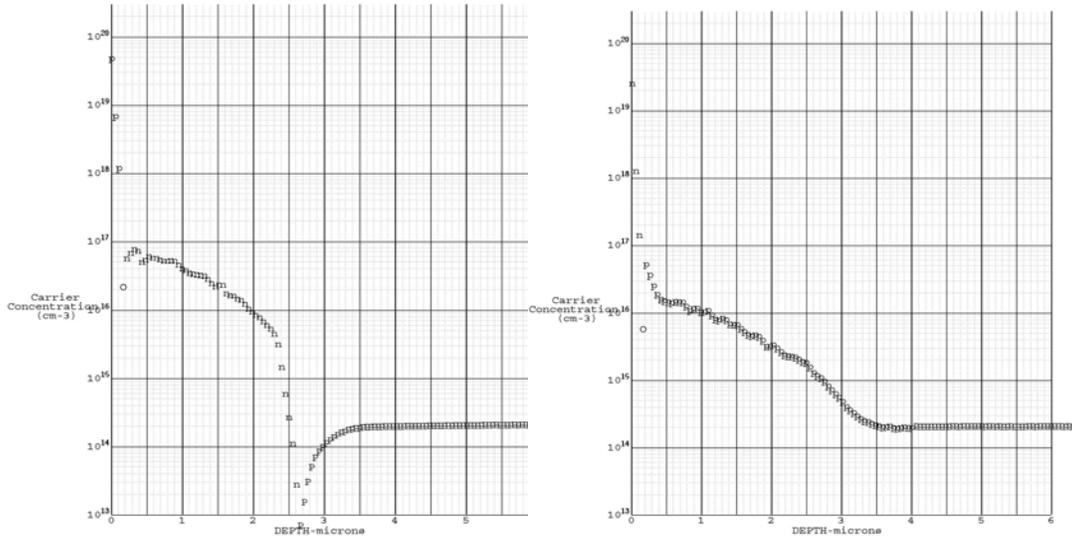
Fig.13 - P-channel (left) and N-channel (right) doping profile under the gate oxide
