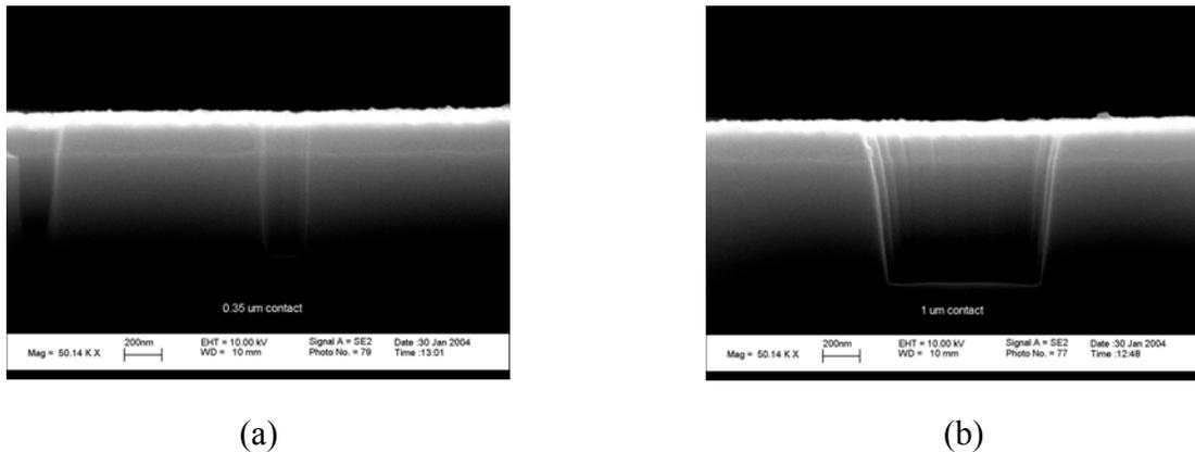
Fig. 2 - SEM cross section of 0.35 μm (a) and 1 μm (b) contact holes etched in 1.5 μm thick LTO
