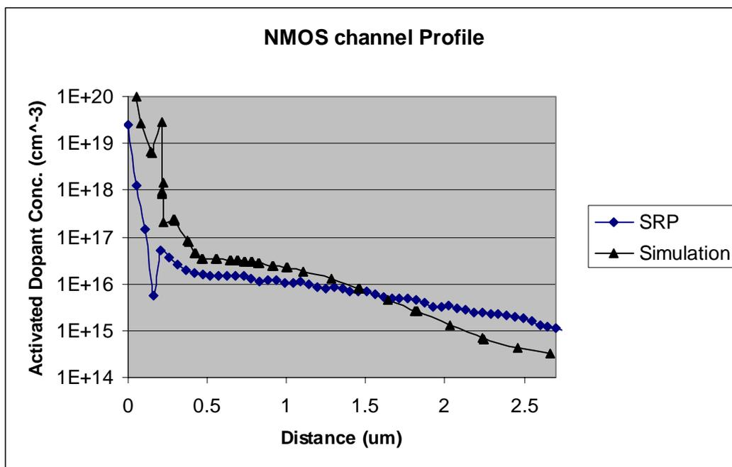
Fig. 9 - Simulated NMOS channel doping profile vs. SRP result
