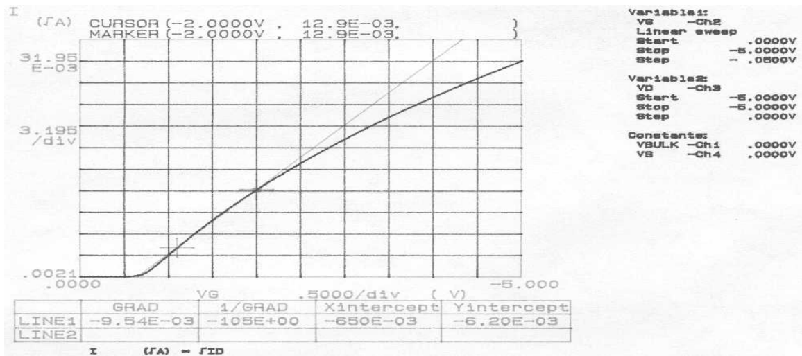
Fig 15. PMOS (W/L=10/1) drain current vs. gate voltage in saturation mode.
