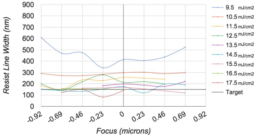
**Exposure Latitude Plot: UV210-0.3 with NA = 0.6 Outer = 0.755 Inner = 0.450**
