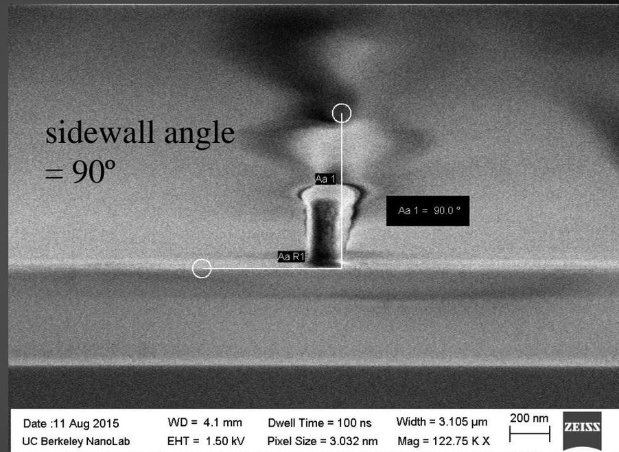
Imaging conditions: 16 mJ/cm<sup>2</sup>, -0.23  $\mu$ m, NA=0.6 Sigma Outer=0.855 Sigma Inner=0.55
