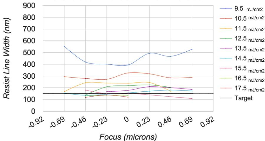
**Exposure Latitude Plot: UV210-0.3 with NA = 0.6 Outer = 0.855 Inner = 0.550**
