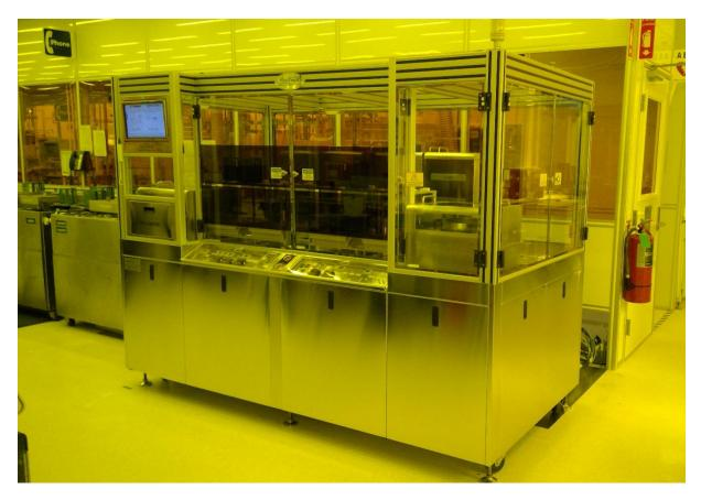
Fully automated coat R&D scale dual 6" and 8" coat and develop track.
