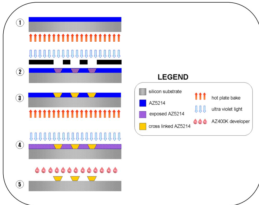
**Figure 18.3 - AZ5214 Single Layer Method Process Flow**
