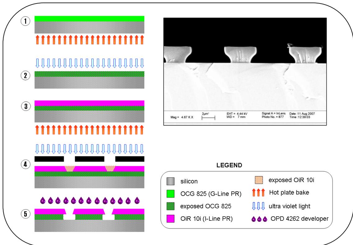
**Figure 18.2 - G-line I-line Bilayer Method Process Flow**
