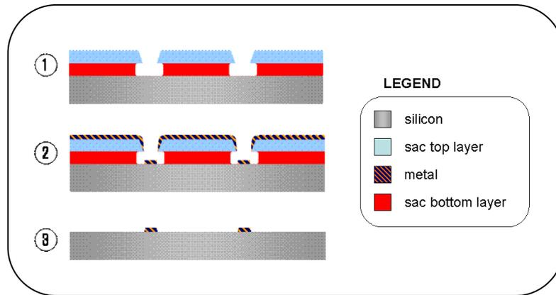
**Figure 18.1 - Basic Lift-Off Process Flow**
